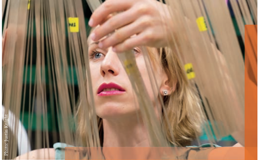
Assistant Professor Polina Anikeeva examines a batch of fiber templates that will be extruded to form tiny opto-electronic neural probes.
